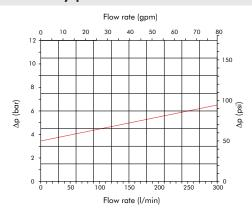
The above diagrams have been obtained at the FILTREC laboratory, according to the ISO 3968 specification, with mineral oil having 30 cSt viscosity and 0,86 Kg/dm3 density.
