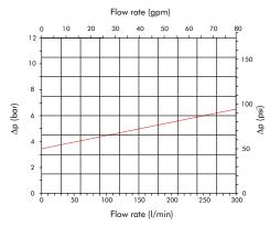
The above diagrams have been obtained at the FILTREC laboratory, according to the ISO 3968 specification, with mineral oil having 30 cSt viscosity and 0,86 Kg/dm3 density.
